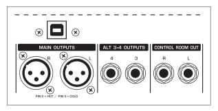
Fig. 2.14: Main mix outputs, Alt 3-4 outputs and control room outputs
